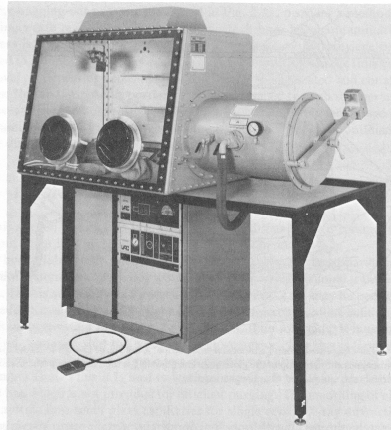
Fig. 2.13. Commercial metal glove box. An aluminum glove box with a recirculating gas-purification system. (Reproduced by permission of the copyright owner Vacuum Atmospheres Corp., North Hollywood, Calif.)
