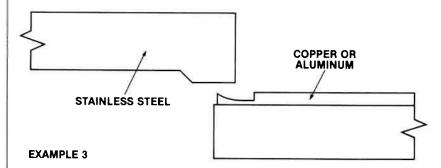
Example 3 is still another improvement of the metal-seal design. The relatively thick main body of the gasket helps to provide a capturing effect. Also, positioning errors are not so critical, and the life of this design is extended. The valve can be baked to 400°C in the open position. However, no bakeout specifications are published for the closed position.
