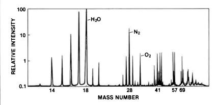
In this illustration, we can see that the vacuum system has an air leak by the large amount of nitrogen, oxygen and water vapor shown in the display. The instrument can then be used to find the leak by switching to detect helium only, and the system is probed with helium. When the probe is placed near the leak, helium enters the system and is quickly displayed. This pinpoints the location of the leak. Other gases may be used to probe for leaks if the RGA is properly tuned to that gas.
