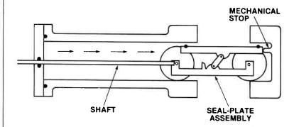
During the forward motion, grease and other debris get into the vacuum environment. And, the longer the stroke, the greater the contamination.
