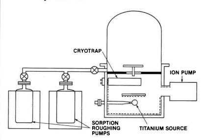
Sorption pumps are very clean. They have no moving parts and do not use oils in their operation. For this reason, they are typically used in ultrahigh vacuum systems. This system configuration includes sorption roughing pumps, a titanium sublimation pump, and an ion pump.
