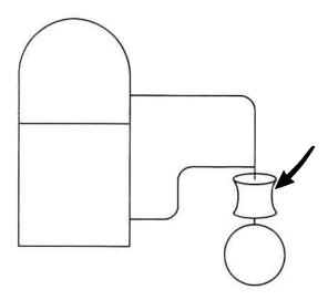
Hoses should be used as convenient couplings, not as long tubulations. In any case, the hose walls should be thick enough so that they will not collapse under a 15 psig pressure differential. When kept in inventory, hoses should be capped or kept in plastic bags so they will not soak up water vapor during their shelf life. Tygon is generally recommended. Also, overly tight hose clamps can cause leaks.
