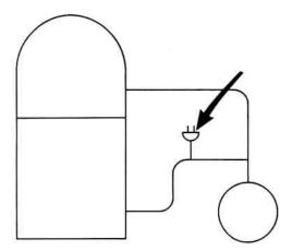
It should be recognized that a foreline TC gauge is especially subject to oil contamination. Therefore, it is more apt to fail or give incorrect readings sooner than TC gauges located in other parts of the system.
