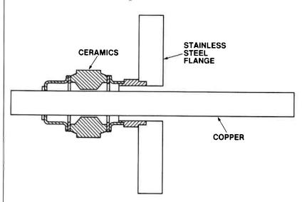
This feedthrough has a large-diameter copper rod that makes it good for high current loads. In fact, the hefty 5/8 in. copper rod conductor makes it seem pretty sturdy. But it is really not strong at all. This is because the entire weight of the copper rod is supported at a single point that also happens to be a vacuum seal.
