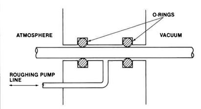
**VALVE WITH DOUBLE O-RING SEAL**
