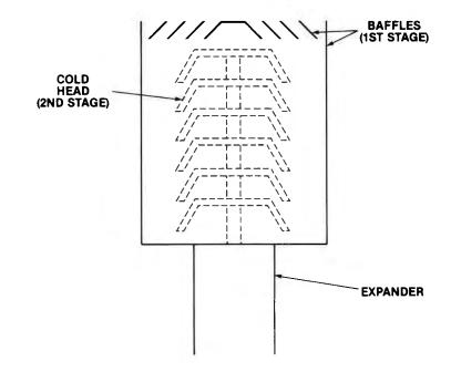
To keep the charcoal surfaces available for the harder-to-pump gases, the outer surface of the cold head is left uncoated. This provides adequate surface on which to condense the easy-to-pump gases. The charcoal is therefore less accessible to the easy-to-pump condensable gases. Finally, a baffle or first-stage cryo-array is placed around the cold head to limit the conductance to the charcoal surfaces.
