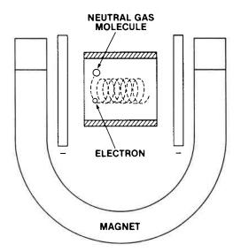
A dc voltage of about 2,000 volts attracts electrons in the gauge tube to the positively charged anode. The magnetic field forces the electrons into long helical paths. This increases the probability of electron-molecular collisions. The collisions produce ions. This, in turn, produces a glow discharge.
