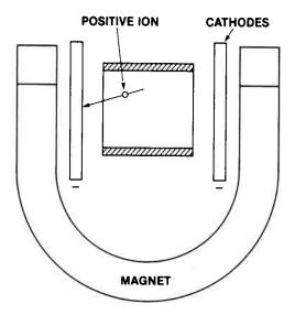
The positive gas ions are now attracted to the negatively charged cathode. The resulting ion current is measured and calibrated in units of pressure. (Note the similarity between this gauge and the ion pump—the cold cathode gauge is an ion pump with nongettering cathode material.)
