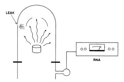
For example, coating material builds up with time, outgasses and raises the pressure. The RNA can tell the difference between outgassing, which may be still within acceptable limits, and an air leak, which is not.
