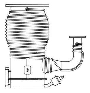
The diffusion pump will not operate at or exhaust to atmospheric conditions. It begins to work at  $10^{-3}$  torr, after the mechanical pump has exhausted most of the air. It therefore must have a backing pump, or forepump, to operate. It, like other high vacuum pumps, cannot successfully operate at atmospheric pressure.
