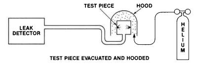
The second outside-in technique consists of hooding the test piece with something like a plastic sheet or dome and flooding the hood with helium as shown. This technique has two obvious advantages. First, it helps to quickly establish whether or not a test piece leaks. Secondly, it establishes the total leak rate. That is, the problem may be the result of a number of very small leaks. Each of the leaks may not individually constitute a problem. But
