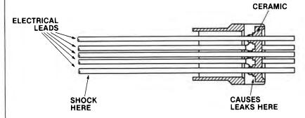
The more electrical leads on a feedthrough, the greater the chances for leaks to develop.
