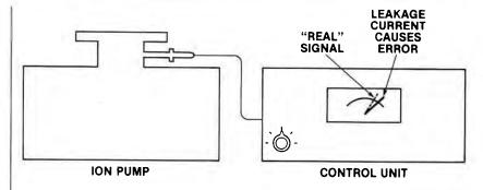
The leak paths may not be dead shorts, but they can cause error signals. An error signal may add to the true signal, and incorrectly indicate high pressure. This can lead to lost time searching for vacuum leaks that don't exist.
