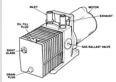
The pump module is immersed in an oil bath. This oil is purified to remove high vapor pressure contaminants. The oil serves the following purposes:
