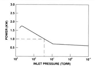
The power requirement at various inlet pressures (or, in other words, at various flow rates) is shown above. The shape of the power curve depends on specifics of design, such as stage matching and the interstage exhaust valve system, but the general relationship is not unlike the one obtained with the conventional pumps. The peak demand occurs typically anywhere between one third and one atmosphere, depending on design.
