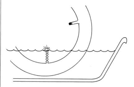
The bubble test is a commonly used method of locating a leak in a bicycle tube. A bicycle inner tube leak that releases a steady stream of very small bubbles releases about 1 std cc of air in 10 seconds. In leak detector terms, this is about equivalent to a  $10^{-1}$  std cc/sec leak rate.
