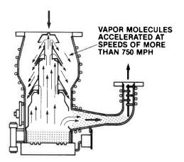
These vapor streams are directed toward the outer walls of the pump. The walls are typically cooled by water. When the vapor hits the cooled walls, it condenses back into a fluid. This fluid then flows downward into the pump boiler for reboiling.
