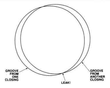
This drawing shows how the knife edge grooves can produce vacuum leaks where the grooves crisscross if the seal-plate position isn't exactly maintained. If the grooves do crisscross, a leak can be avoided by using greater sealing pressure each time a closure is made. This limits the life of the gasket, however.
