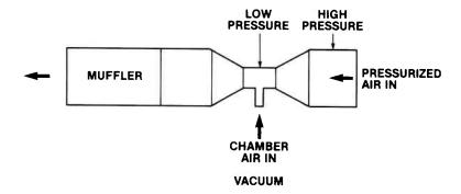
A Venturi pump is simply a tube with a pinched midsection. The tube has an inlet from the work chamber, a pressurized air inlet, and an exhaust. A muffler at the tube exhaust reduces the noise level during pumpdown.
