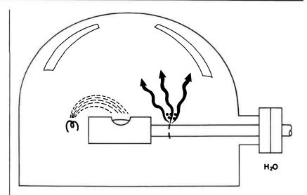
There are real leaks which act like virtual leaks. An example is a cooling line leak which "looks" like a virtual leak because it is not directly connected to the outside.
