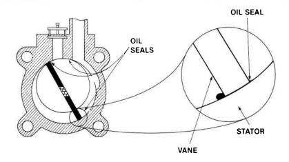
A thin film of oil makes the final seal in these pumps. Therefore, base or ultimate pressure is partly determined by the vapor pressure of the oil. If the oil becomes loaded with water, or other impurities, these contaminants increase the vapor pressure. Then it is impossible to reach satisfactory low pressures. The oil is a very important part of your mechanical pump. Dirty pump oil is usually the reason why the pump is not performing well.
