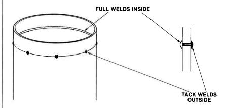
When the full weld is made from the inside but an outside weld is desired for structural strength, the outside weld should be a tack weld, not a complete weld. This makes leaks easy to find and fix. It also prevents virtual leaks that occur because of a trapped volume between the two weld joints.
