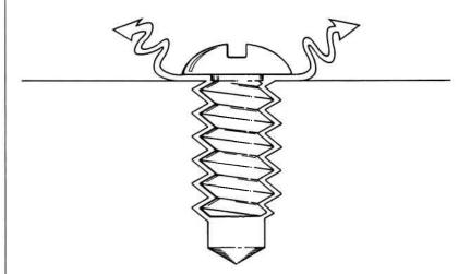
Virtual leaks, which we have already discussed, can be the cause of excessively long pumpdown times, if not complete system failures.
