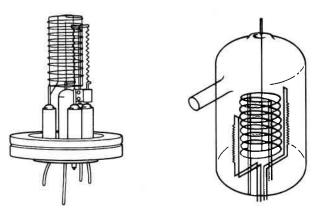
The ionization gauge is perhaps unique in that it can be used over a pressure range spanning eight orders of magnitude ( $10^{-3}$  to  $10^{-11}$  torr). It is commonly used over seven orders of magnitude ( $10^{-3}$  to  $10^{-10}$ ) and expected to be within  $\pm 20\%$  of the correct value over that range. This makes it the most widely used gauge for high vacuum work. Models include both glass and metal envelopes as well as "nude" gauges which mount directly in the chamber.
