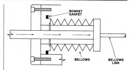
BELLOWS ACTUATOR ELIMINATES O-RING ROLLING, SCUFFING
