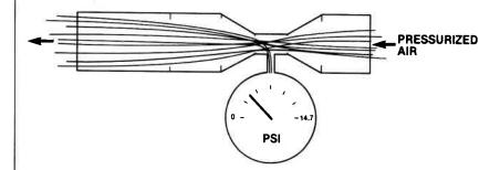
Pressurized air at about 60 psig entrains air from the work chamber and exhausts it through the noise muffler. The chamber is evacuated to about 60 torr, then a sorption pump continues rough pumping. It's a very rough roughing pump, but it does offer this advantage:
