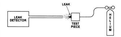
inside-out leak detection technique
