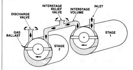
Gases from the chamber enter the inlet port. They are swept around by vanes, and compressed. Compression builds up pressure to overcome atmospheric pressure. The spring-loaded discharge valve is opened. The air is then expelled to atmosphere. These pumps can remove over 99.9% of the air from the chamber.
