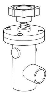
These valves use various elastomers to make a reliable, leak-tight interface between the valve seal and the seat. Elastomers are also sometimes used to seal the actuating shaft from the outside environment.
