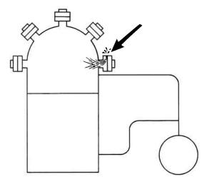
In modern industrial vacuum systems containing many feedthroughs, there are many opportunities for leaks to occur. You can see an example of a leaky flange in the illustration above.
