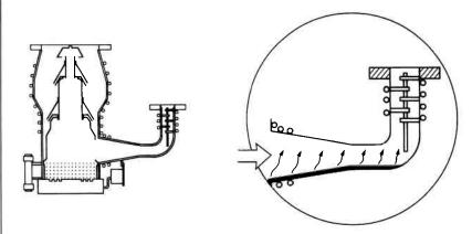
In addition to the vertical jet assembly, modern pump designs incorporate an ejector stage. This stage helps to move gas molecules out of the pump body and into the foreline. This action allows higher pressures in the foreline, which in turn allow the mechanical forepump to efficiently remove the compressed gas molecules. Pumps with ejector stages usually have a baffle in the foreline to prevent oil vapor loss to the forepump.
