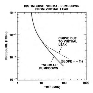
The pumpdown curves are also very useful for distinguishing normal pumpdowns from problem pumpdowns; in this case, from a problem due to a virtual leak. Notice how the normal pumpdown curve is compared against a virtual leak pumpdown. Notice how the virtual leak pumpdown curve shifts rather dramatically.
