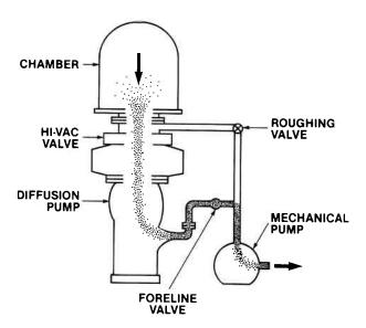
If an operating diffusion pump is exposed to atmosphere for any length of time, severe oxidation or breakdown of the fluid can occur. Sometimes, in extreme cases, a fire or explosion in the pump may result. The contaminants created in these cases will severely hinder pumping speed and operation due to the gas loads they will contribute to the system. A diffusion pump at atmospheric pressure acts just like a pan of hot oil on a stove. Leave it too long—it will thicken, harden or burn!
