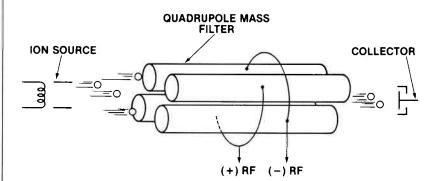
The residual gas analyzer separates, identifies and measures the partial pressures of residual, or remaining, gases in an evacuated chamber. The gases produce peaks in the display. The position of the peaks identifies the gases producing them. The partial pressures of the gases are measured by the heights of the peaks. Total pressure can also be measured.
