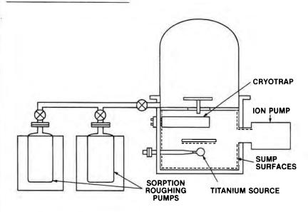
Typically, UHV systems require an ultraclean environment. Because of this, TSP pumping is often used together with ion pumps and  ${\rm LN_2}$  traps or baffles. These systems are usually rough pumped by sorption pumps.
