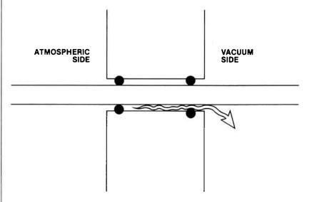
Virtual leaks can also result from double O-ring-sealed shafts.
