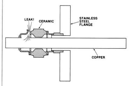
This means that the feedthrough is not intended to support any weight or to withstand any torque forces or shocks. The feedthrough is designed for electrical conduction only, and not for mechanical support.
