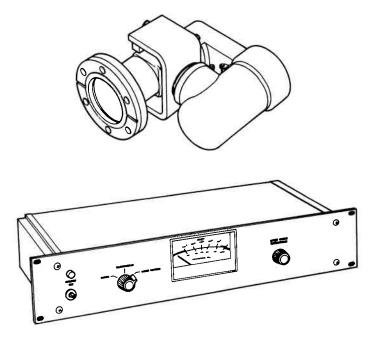
The residual nitrogen analyzer (RNA) reads the total pressure and the nitrogen partial pressure. It operates in the high vacuum range.
