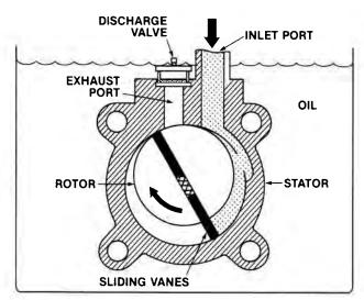
**ROTARY OIL-SEALED MECHANICAL PUMP MODULE**
