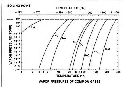
Most gases are condensed on the first- and-second stage cryoarrays. The first-stage array is cold enough to pump water vapor by cryocondensation. The second-stage array is cold enough to pump nitrogen, oxygen, argon and most other gases by cryocondensation.
