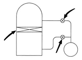
Valves can malfunction. Wear, caused by high friction forces, can prevent proper sealing. The seals wear in time. The actuating air pressure on pneumatic valves may be too low to provide proper sealing. Solenoids may be faulty.
