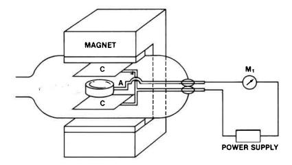
A cold cathode gauge consists of a gauge tube and control unit. The gauge tube has a central anode and two cathodes or a cylindrical cathode. A strong permanent magnet surrounds these elements. Its accuracy is approximately  $\pm 50\%$  of the true pressure.
