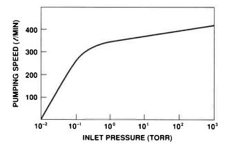
The basic pumping performance of the dry pump is shown in the form of a traditional pumping speed curve. The shape of the curve is very similar to the typical curves obtained with oil-sealed pumps. The gradual decline in speed toward the lower pressure is due to the changes in volumetric efficiency and the switching of the flow from the regular valves to the inlet slots. The final decline toward 10 mtorr is due to residual leakages which produce the limiting compression ratio.
