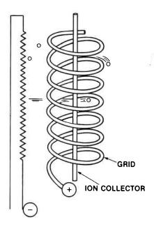
Let's look at the process in more detail. Electrons emitted by the hot filament are attracted to the positive grid. However, many electrons miss the loosely wound grid and swing past it several times before finally striking it. Because of the large number of electrons emitted by the filament, a fairly constant "electron cloud" is present about the grid in the gauge tube.
