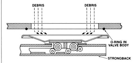
The conical shape of the seal plate causes process debris to fall away from the seal area. Also, the seal is located in the valve body instead of in the seal plate. This location further minimizes the possibility of seal leaks.
