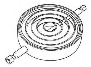
Baffles, however, make a useful contribution to the effectiveness of diffusion pumps. (Refer to the chart titled "Backstreaming" in the Diffusion Pump section to see how baffles can reduce diffusion pump backstreaming.)
