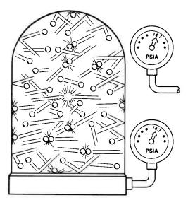
As air is pumped out of the chamber, pressure drops. However, we can never remove all particles from the chamber.
