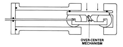
The valves are often air-operated and close with considerable speed and force. It is important to remember to disconnect both air and electricity when working on them.
