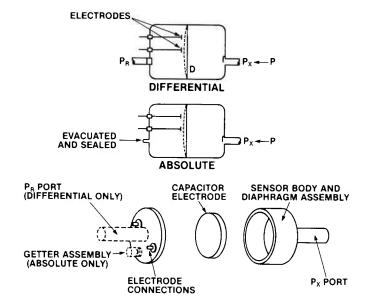
The diaphragm deflects with changing pressure—force per unit area—independent of the composition of the measured gas. This causes a capacitance change between the diaphragm and the adjacent electrode assembly. The capacitance change is sensed in an oscillator circuit and converted to a frequency change proportional to the diaphragm deflection.
