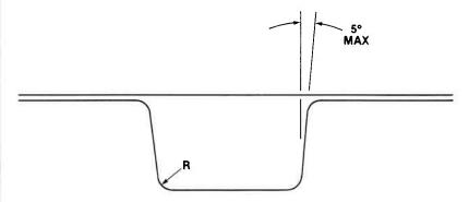
The groove in the flange for the O-ring should have sides that slope outward to a maximum of 5°. The groove should also have a radius on the inner corners equal to about two-tenths of the O-ring diameter. The surface finish of the seal area should be at least 32 microinches. The outer edges should be smooth, to avoid scratching the O-ring when making the seal.
