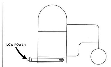
When replacing heating elements, be sure to tighten the elements, the clamps, and the crush plate to provide good intimate contact and good heat transfer. Also, make sure that the proper heating element is used. Check the voltage rating on the replacement element before installing it. If a crush plate is used, replace it with a new one when you replace the element. If wires or wire lugs must be replaced, they must be the nickel wire and lugs provided by the pump supplier.
