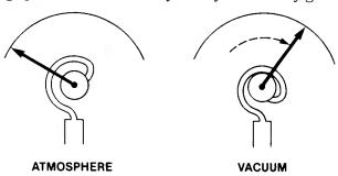
The inside of the tube is open to the chamber, and the outside is at atmosphere. As the chamber is pumped out, the pressure difference between the inside of the tube and the outside of the tube causes the curvature of the tube to change. A system of levers and gears moves the needle according to the change in the bend of the tube.
