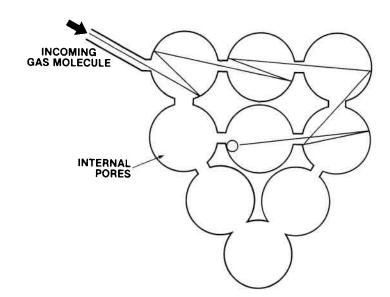
Cryosorption is the trapping of gases not readily condensed or pumped at  ${\rm LN_2}$  temperature. Cryosorbed gases are trapped in the pump's molecular sieve material.
