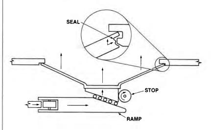
SEAL PLATE MOVING INTO SEALING POSITION
