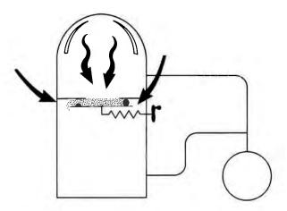
Debris, particularly at the valve seals, is quite often the cause of system failure. Bellows or other feedthrough devices can leak. Double O-ring shaft seals can be the sources of virtual leaks.
