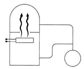
The liquid nitrogen trap should never be allowed to go dry while the high vacuum valve is open. This is sometimes mistakenly practiced on weekends when the system is on standby. However, as the  $\mathrm{LN}_2$  trap warms up, it releases all the trapped gases, particularly water vapor, that it had captured during the work week. A significant amount of water vapor and other contaminants are then free to go back into the work chamber.
