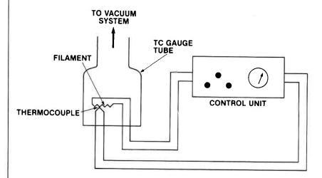
A thermocouple gauge consists of a gauge tube and control unit. Within the gauge tube is a heated filament. Spot welded to the filament is a thermocouple that measures the temperature of the hot wire. The meter is calibrated in pressure units, not in temperature.
