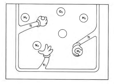
Chemically, titanium is a very reactive substance. The deposited film combines readily with many gases, changing them into solid compounds such as titanium hydrides, oxides and nitrides. This is a form of chemical pumping. When the film of titanium becomes saturated, a fresh film is deposited, and the chemical pumping action resumes.
