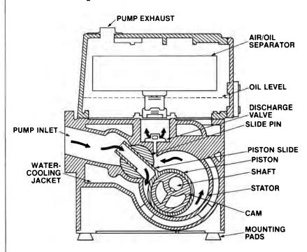
As the eccentric cam turns, it rotates the piston inside the stator. Thus, gases that come in through the sliding valve are compressed by the piston and forced out through the discharge valve and exhaust port. At first, this may seem to be a complicated way of doing things. In fact, however, this is one of the most rugged of the industrial vacuum pumps. Properly maintained and used,
