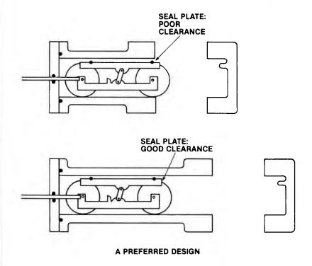
A preferred design completely clears the ports.
