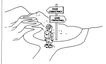
In molecular flow, a good conductance path is wide and short. It has few turns, thus allowing free gas flow. In viscous flow, these conditions are not so important. This is because the molecules tend to push one another along under the influence of a pressure difference.
