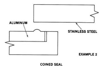
In example 2, an aluminum gasket with a ridge is pressed against a flat stainless steel seat. This is in effect a coined seal. There is enough capturing in this design to produce good seals. Also, this type of seal is insensitive to position repeatability (providing the aluminum is soft enough to avoid denting the seat, and the seat is flat and smooth). However, this capturing effect is lost under high-temperature conditions, especially when the valve is in the closed position.
