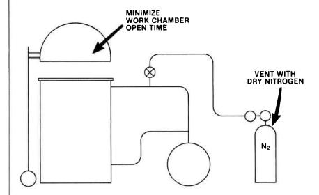
The time that the work chamber is left open and up to atmosphere should be reduced as much as possible. Five minutes is not unreasonable. When many work pieces are processed per cycle, they generally are mounted on fixtures of some kind. By having spare work-piece holders on hand, it is possible to greatly reduce the chamber open time.
