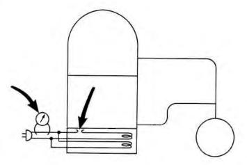
A clamp-on ammeter will establish whether the correct current level is being delivered to the pump. Although an ohmmeter resistance check might seem easier, particularly on single-element heaters, an ohmmeter check can overlook power-robbing, corroded terminals. Resistance is a poor indication of heater condition except for an open heater circuit.
