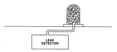
This technique, of course, does not pinpoint the site of the leak; however, it quickly establishes whether a leak (or leaks) exist(s).
