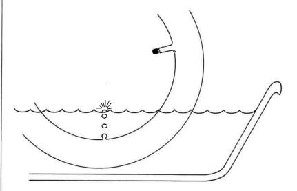
A bicycle tube leak that releases one bubble per second will release a total of 3 cc of air per hour. In leak detector terms, this is about a leak rate of  $10^{-3}$  std cc/sec. A leak rate of  $10^{-4}$  std cc/sec
