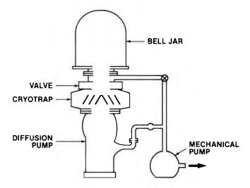
Typically, cryotraps are teamed with diffusion pumps (or other high and ultrahigh vacuum pump systems). Cryotraps have also been used in roughing lines to minimize mechanical pump oil migration toward the chamber. In addition, they have been used with helium leak detectors for the same purpose. For these applications, however, a molecular sieve trap is usually better.
