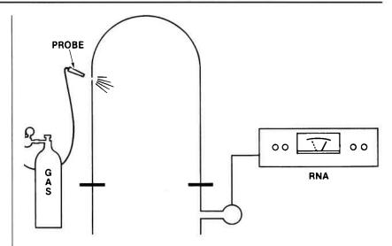
The RNA also can be used to pinpoint the location of a leak. When a gas probe using any gas except nitrogen passes over the leak, the percentage of nitrogen is again changed. This change can be used to establish the location of the leak.
