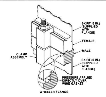
This flange is used for larger diameter seals. It seals by forcing a copper wire into a compressed area under pressure, much like the ConFlat flange. The force is applied with large C-clamps. Wheeler flanges may be used reliably up to 450°C.
