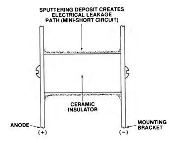
Now let's look at another possible problem, and see how it is handled. We saw in the pump section how gases are ionized by applying a high voltage across a cathode and an anode.
