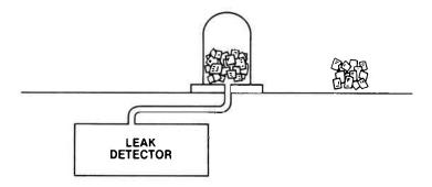
IF LEAK IS INDICATED, REMOVE HALF THE TEST PIECES, AND RETEST.
