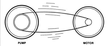
A very loose or broken drive belt can prevent a mechanical pump from operating at all. A loose drive belt might be heard slapping against the belt guard. On a single-belt drive, a broken belt will bring the pump operation to a halt; a broken belt in a multiple-belt drive unit may not be so obvious. A loose belt may not be turning the pump module at the rated speed, thus causing longer pumpdown times.
