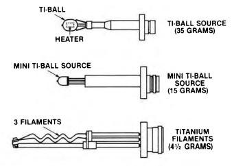
There are various titanium sources. Varian manufactures a three-filament source, a Ti-Ball Source, and a mini Ti-Ball Source. The Ti-Ball Source produces about 750 watts of heat at full power and 200 watts on standby power; the other two sources produce about 380 watts at full power. The mini Ti-Ball standby power is 95 watts; the filament source is simply turned off when not operating. The heat radiated to nearby surfaces may cause excessive outgassing in small volumes.
