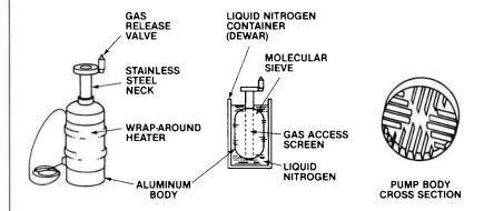
The sorption pump has an aluminum body with internally extruded heat transfer fins (see cross section). The pump is filled with a very porous material known as *molecular sieve*. A pressure relief tube is mounted on the connecting flange. The pump is placed in a dewar containing liquid nitrogen  $(LN_2)$ .
