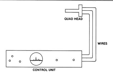
One type of residual gas analyzer includes a quadrupole sensing head and control unit. The control unit has a computer-controlled screen that displays the ion current signals of the gases remaining in the chamber. Some of the older units use an oscilloscope to display the signals.
