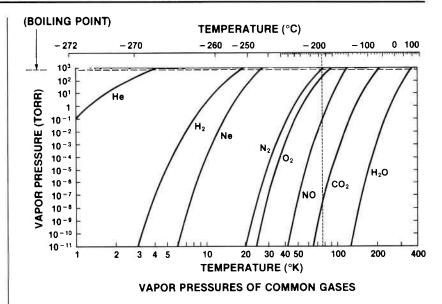
When gases become cooled sufficiently, they liquify and/or freeze. These curves give the vapor pressure for selected gases when they are liquids or solids. Curves to the right of the vertical dotted line  $(77^{\circ}K, -196^{\circ}C)$  indicate low vapor pressures at this temperature. Curves to the left show high vapor pressures at this temperature, which is the boiling point of liquid nitrogen.
