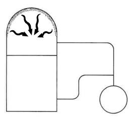
Outgassing, which may be considered to be a virtual leak, can also cause long pumpdown times. In production systems, long pumpdown times reduce the amount of work that can be produced by the system. Outgassing can also seriously affect the quality (yield) of the work. Simple outgassing can be often corrected by systematic, scheduled cleaning procedures.
