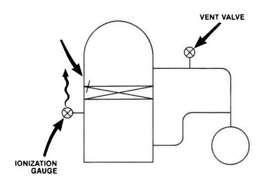
If the pressure goes up (indicated on the ion gauge below the high vacuum valve, if you have one) when the system is vented, this is an indication of a high vacuum valve sealing problem. The pressure should not rise even slightly. There could be dirt, debris, hair on the seal, improper adjustment of the high vacuum valve, or insufficient sealing pressure. The foreline TC gauge can also be used for making this check; however, it is not as sensitive as an ion gauge below the high vacuum valve.
