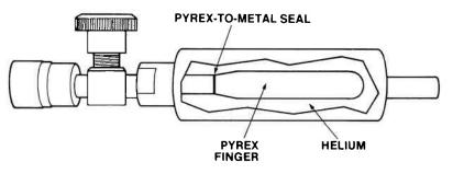
PERMEATION LEAK WITH RESERVOIR AND VALVE
