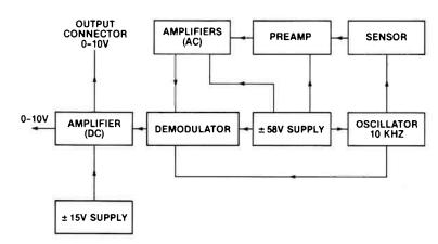
This frequency change, in turn, is converted in the unit to be displayed as the pressure reading. The sensor unit may be constructed of materials such as inconel and stainless steel, allowing the gauge to be used with corrosive gases.
