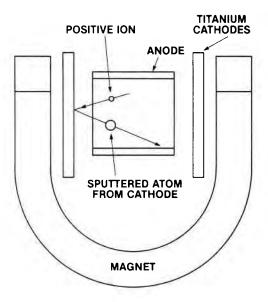
The positively charged ions, which are relatively heavy particles, are accelerated into the negatively charged titanium cathodes. This impact causes sputtering, or chipping away of the titanium cathode material.
