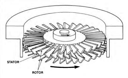
The turbo pump is mainly composed of rotating and fixed disks. These are called rotors and stators, respectively. The rotor disks are arranged alternately with the stator disks. On each disk are blades. A disk may have from 20 to 60 blades. The number of blades on a disk, the blade length, width, spacing and rotational speed determine its ability to pump gases.
