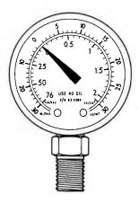
The Bourdon gauge is rugged and reliable. It can be used for measuring pressures above and below atmospheric pressure. Notice that it resembles a vacuum pressure gauge used in automotive tune-ups—same principle!
