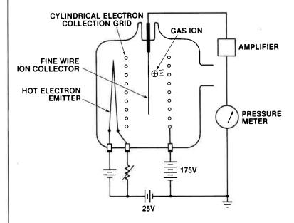
The positively ionized gas molecules are attracted to the collector. This produces an ion current proportional to the pressure in the chamber. To get meaningful pressure readings, the sensitivity of the gauge must be known, and the emission current must be well regulated. The "sensitivity" selector on the controller must be set the same as the rated sensitivity of the gauge tube. If this "matching" is not done, you will get inaccurate pressure readings.
