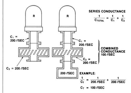
Let's look at the result (point "R" at the vacuum chamber) of adding a pump (shown in the drawing) with a speed (S) of 200 \(\ell\)/sec to the combined 100 \(\ell\)/sec series conductance.
