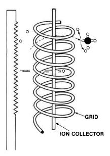
On their long, round-about flight to the grid, electrons may collide with gas molecules, ionizing them and releasing more electrons. The longer the flight of these electrons, the greater the chance of collision. Therefore, a stronger, more usable signal is produced.
