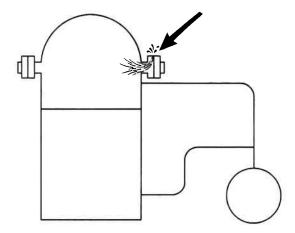
Leaks certainly are a major reason for system malfunctions. Air leaks are not uncommon. If small enough, leaks of this type can be ignored in many processes. (We'll consider sizes of leaks, or leak rates, in the Leak Detection chapter.)
