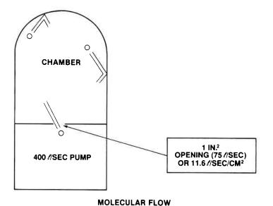
In the molecular flow range, a 1 in.<sup>2</sup> opening has a 75  $\ell$ /sec conductance. The pump speed, in this case 400  $\ell$ /sec, is really 75  $\ell$ /sec as far as the chamber is concerned because the mole-
