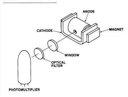
The RNA is a cold cathode gauge that also includes a window, an optical filter, and photomultiplier tube. Ionization produces light. This light has various colors, depending on the gases producing it. The filter passes nitrogen light and blocks the light from other ionized gases. Thus, the gauge reads only the nitrogen pressure. In the "normal" mode, this cold cathode gauge also reads the total pressure. We can use this to help us in determining the condition of our vacuum system.
