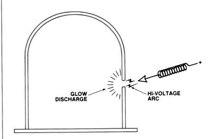
The spark coil technique uses a high-voltage or tesla coil to create an arc. This causes the ionization of air at the point where it enters the system. Ionization, of course, creates a glow discharge which is visible in glass systems. This is a simple technique; however, it has a number of drawbacks. First, it can only be used in glass systems. Further, this technique is potentially dangerous. (The high-intensity arc could cause an implosion.)
