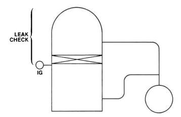
However, the actual problem may not be so simple to solve. Leak checking is one approach to the problem; there are others. A good pressure reading below the closed high vacuum valve might eliminate that part of the system as a problem area.
