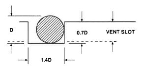
The depth of the groove provides for deformation of the O-ring to about 70% of its unsqueezed diameter. This gives enough elastomer material to make the seal without overstressing the O-ring, but not so much as to force it out of the groove where it might be pinched or cause excessive outgassing. A vent slot is usually machined across the face of the groove to eliminate trapped volumes and for leak detection.
