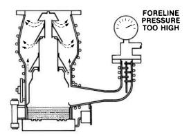
A reduction of the normal pumping speed (actually throughput)—caused, for example, by a reduction in heater power to the boiler—will cause a corresponding reduction of the maximum tolerable forepressure.
