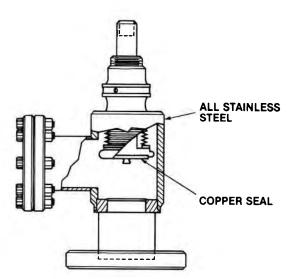
Varian all-metal valves use the gasket-capturing design discussed in the flange section. This insures that the gasket material won't flow away from the seal area, even under bakeout temperatures of  $450^{\circ}$ C.
