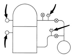
The first indication of a system malfunction is provided by the pressure gauges. However, we must also recognize that the gauges themselves can malfunction, either failing completely, or giving us false information as to the system status. Failure to recognize this fact can lead to the wrong conclusion.
