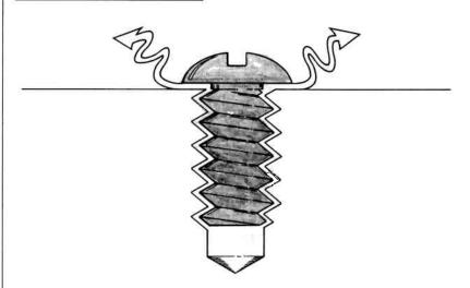
Trapped volumes, also called virtual leaks, are sources of gases that are inside the vacuum system but which are released very slowly into the system. For example, water vapor on the walls, solvent residues, and trapped volumes can release gases into the system over a long period of time. This can make it impossible to reach satisfactory pressures until all of the gas is completely released.
