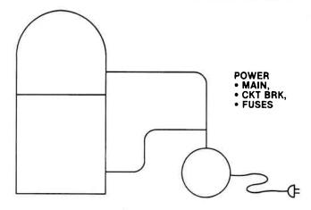
Check the easy things first. Is power arriving at the unit? If not, possibly a circuit breaker has opened. If the system is equipped with fuses, they may be burned out. Also, consider loose or broken connections. A pump or drive motor might be frozen, or seized. This condition might show up as a characteristic whining or buzzing sound as the unit struggles to turn, as overheating, as odor, or as all three of these symptoms.
