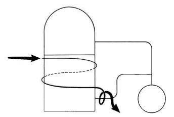
How is the water in your facility? Hard water is full of minerals which, when deposited over a long period of time, can plug (or partially plug) the water lines. This defeats their cooling function. Thirty-five percent muriatic acid and water flushed through the water lines will help to unplug them. Do not use deionized water! Most facilities today use a treated, recirculated water supply. Water filtration and treatment may be a good investment if your area has water problems.
