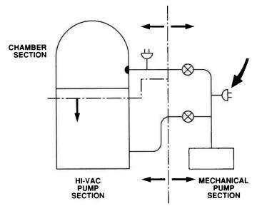
Use of valve isolation and pressure readings to identify cause of poor base pressures.
