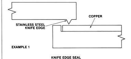
In example 1, a stainless steel knife edge is pressed into an OFHC copper plate. Since the knife edge penetrates the copper gasket, it is essential to reposition in precisely the same location on subsequent cycles. The slightest error in location produces a new groove pattern in the gasket material. This, of course, results in a leak. Leaks can be avoided when positioning errors exist. However, a large increase in sealing force is necessary.
