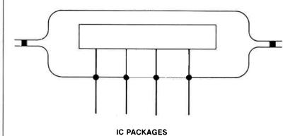
An example of leaks that don't occur in definite patterns can be found in the semiconductor industry. Typically, the average frequency of leakers in production IC packages is 1% to 2% with no observable pattern of size or incidence of leaks.
