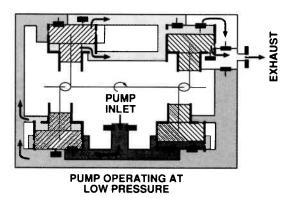
The dry pump has two interstage exhausts and, in addition, the flow into the *last cylinders* is proportioned by controlling the conductances of ducts.
