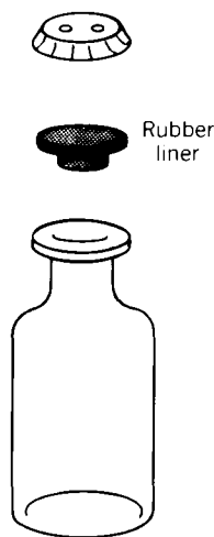
Fig. 1.31. Heavy-walled centrifuge-tube, rubber cap liner, and cap. ("Pop bottle" reactor.) Tubes with volumes ranging from 20 to 250 mL are available from Lab Glass, North West Boulevard, Vineland, NJ 08360.
