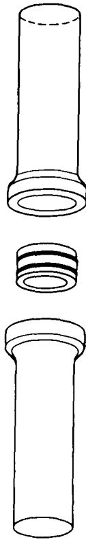
Fig. 8.4. Solv-seal joint. A pair of O-rings form the seal between the Teflon cylinder and glass joints. The cylinder fits inside the glass parts. A compression clamp (see Fig. 8.3c) holds the joint together.
