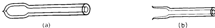
Fig. II.9. Preparation of capillary tubing for an end-to-end seal. (a) A tube blown out to normal wall thickness. (b) The same tube with the end blown out.
