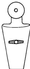
Fig. 8.9. Notched stopcock plug. A triangular file drawn across the orifice at right angles to the length of the plug will notch the orifice. This may then be used to better control gas flow, such as an inert-gas flow while working on a Schlenk manifold.
